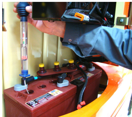
Figure 5-8. Measuring Electrolyte Specific Gravity
